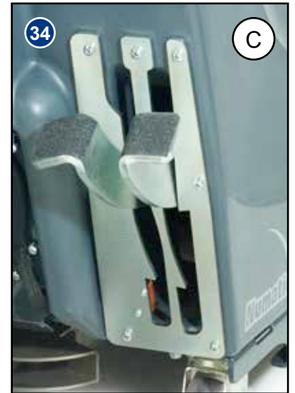
(C) Extra Heavy Scrub 50 Kg Pressure (Fig.34)
